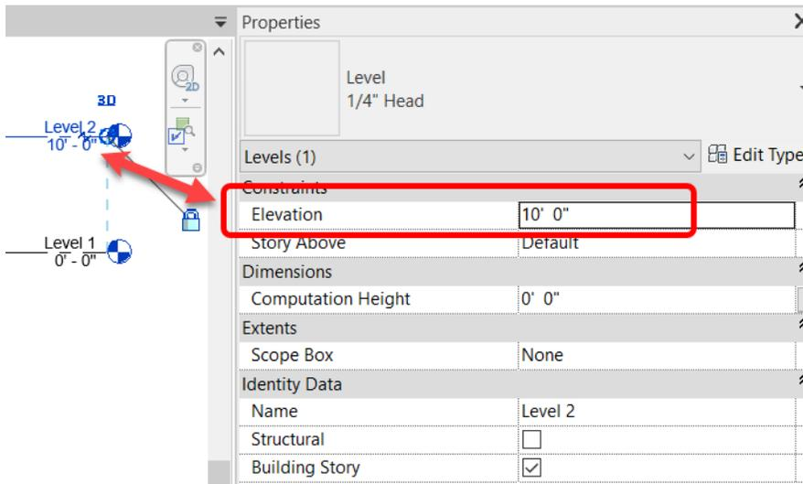
The height indicated can be relative to one of two origin points in Revit. The 'Project Base Point' or 'Survey Point'. To change which origin point the level line is associated with:
