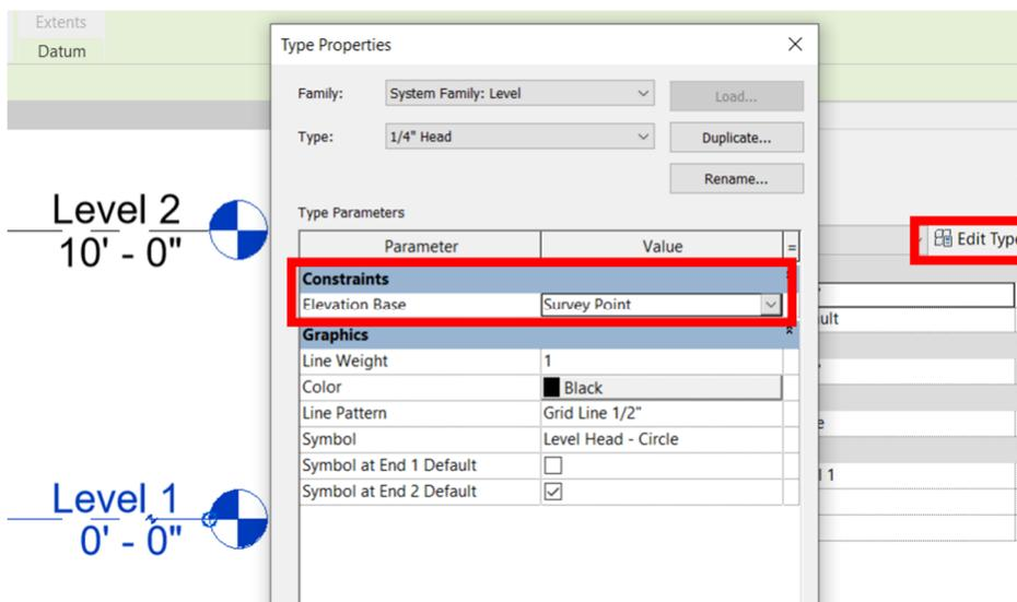
This change will affect all level lines in your project. If desired, you can create duplicate level “types” and create one option for each elevation base, thereby allowing you to reference either base in the same project.
